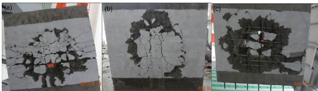
Fig.1. Crack pattern of (a) SS (b) SF and (c) SF0.37P35-0.5 slab
