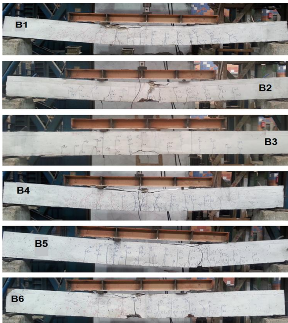
Fig.20. Crack pattern and failure for specimens
